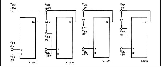
The ADDRESS (digtal-control inputs) and INHIBIT logic levels are : "0"=V<sub>SS</sub> and "1"=V<sub>DD</sub>. The analog signal (through the TG) may swing from V<sub>EE</sub> to V<sub>DD</sub>
